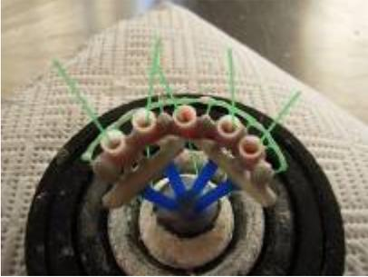
Figure 17 A thin gauge sprue wire is inserted into each cylinder
