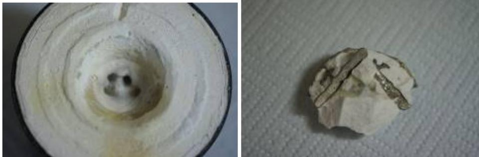
Figures 23 & 24 No casting 'button' is formed, note that the direction of casting force is marked into the investment prior to burn out
