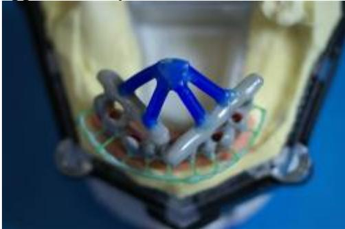
Figure 16 The spruing technique utilises a segmented runner bar to help prevent warpage
