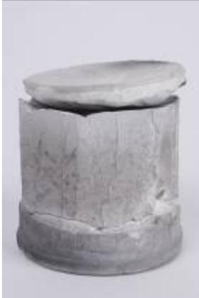
Figure 11 Rapid expansion of plastic components can cause investment material to fail
