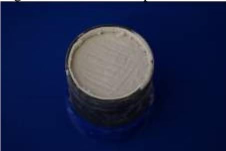
Figure 20 Once set the investment material should be roughened to allow the escape of gases
