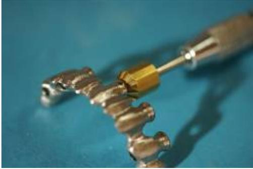
Figure 25 The framework is inspected and any slight imperfections removed
