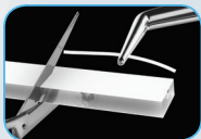
Cut the fibre bundle inside the silicone
